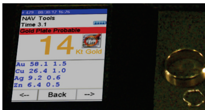
The Niton DXL analyzer's AuDIT feature instantly warns you of the probability of gold plated material
